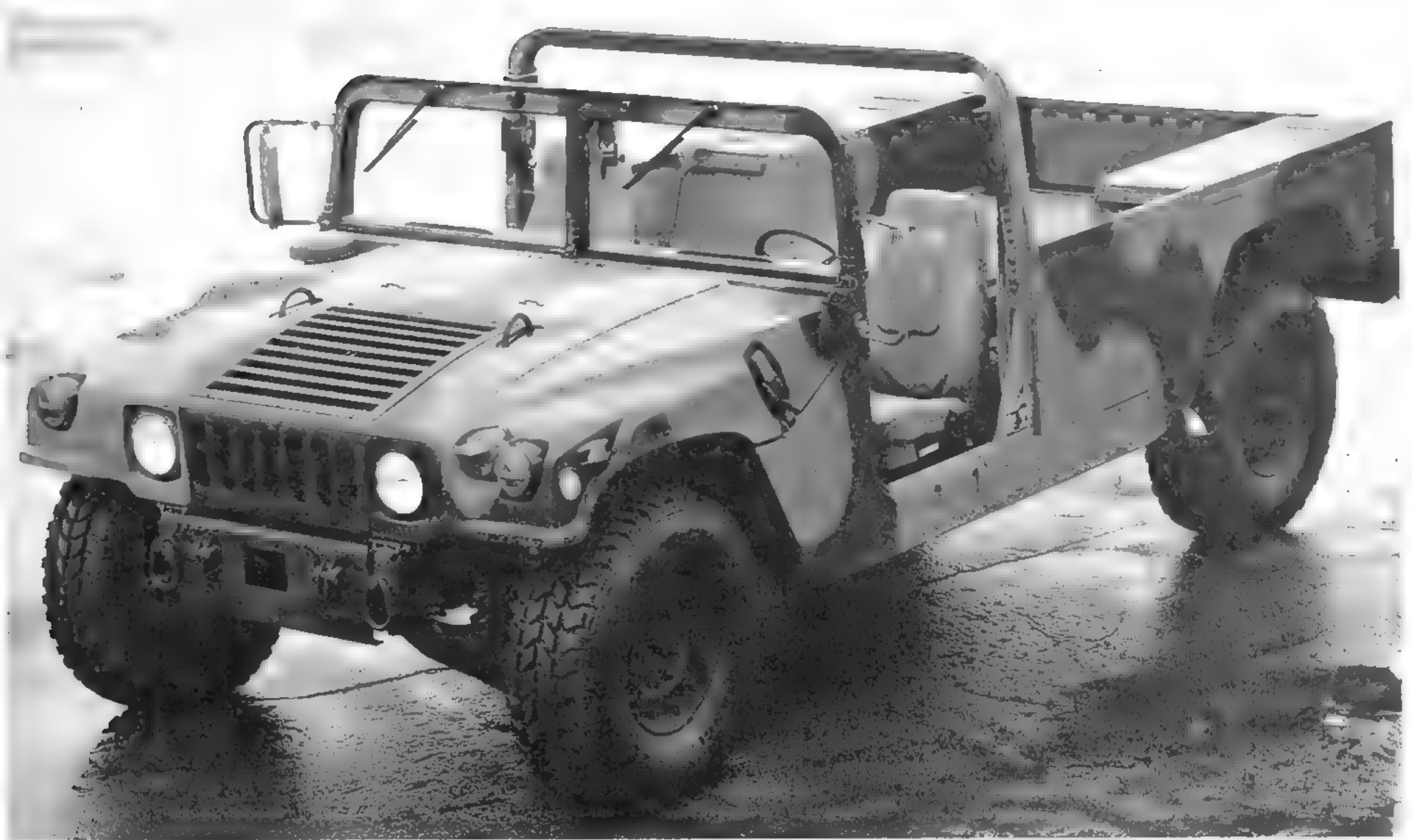
The M998 could also be configured as two-seat pickup truck. This truck lacks the optional brush guard. (Photo courtesy of AM General Corp.)
